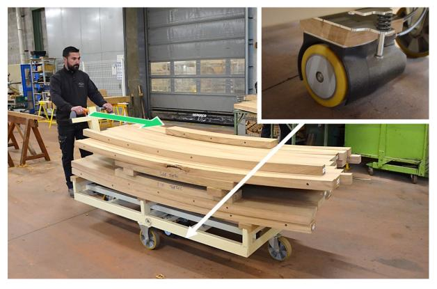
By reducing physical strain, improving ergonomics, and enhancing safety, **AWD®** wheels facilitate compliance with ISO 11228-2. They provide an effective solution for preventing MSDs and improving working conditions for operators.
